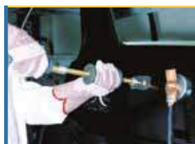
Spot hammer welding
